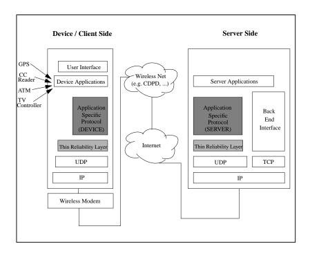
Figure 1: Anatomy of a Vertical Wireless Application
