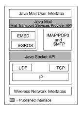
Figure 1: Components of JavaMail Transport Service Provider with EMSD
