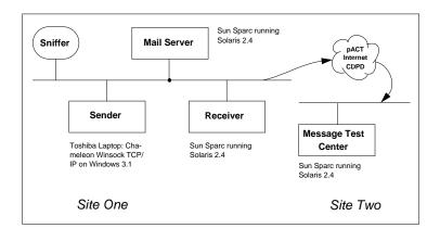
Figure 1: Experimental Setup for Submission
